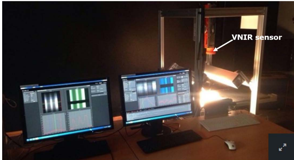
Figure 3-1. The experimental laboratory setup for image data collection. On the tripod in the centre is the VNIR imaging spectrometer camera placed at an angle of 90^{\circ} . Next to the sensor is a sliding table where the soil tray is placed for scanning. On the right and the left side of the sliding table, an external light source is integrated to illuminate the tray during image acquisition.
