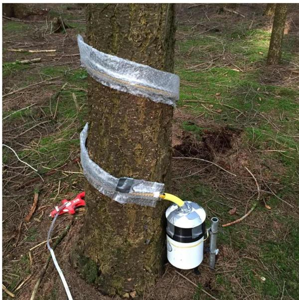
**Figure 2.4** Stemflow measurements in the 'Speulderbos' study site
