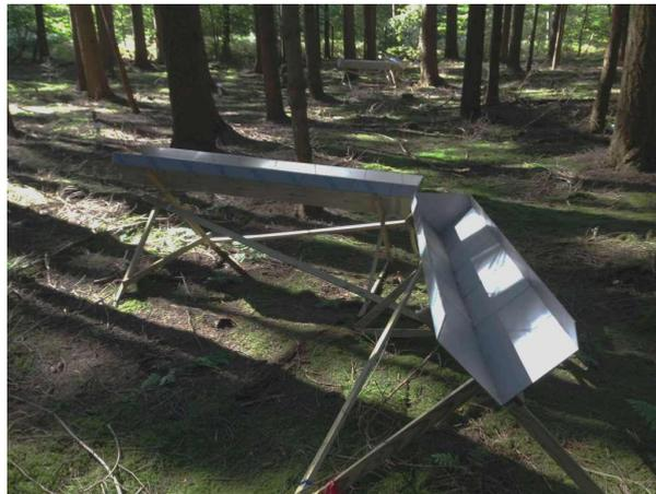
**Figure 2.3** Throughfall measurements in the 'Speulderbos' study site
