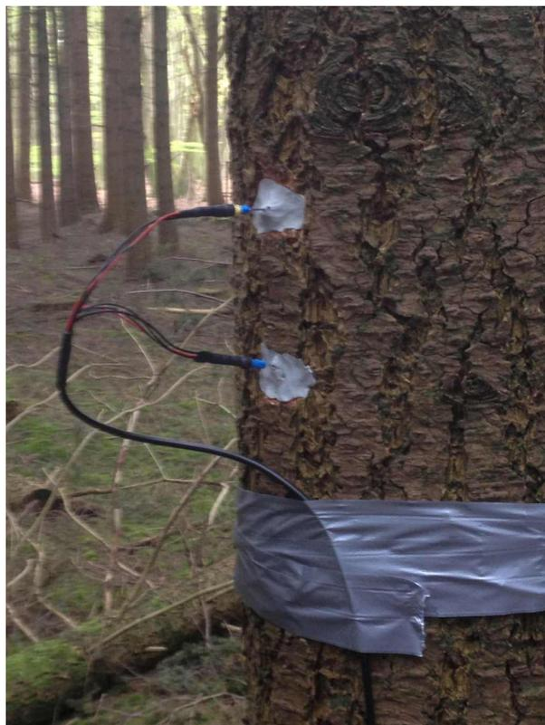
**Figure 2.7** Three thermal dissipation probes (TDP) placed in a Douglas fir stem in the 'Speulderbos' study site
