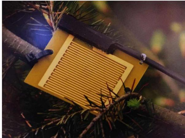
**Figure 2.6** Leaf wetness sensor (Model 237) placed in a Douglas fir branch in the "Speulderbos" study site
