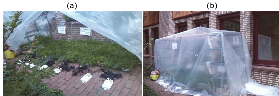
Figure 2.1. Experimental setup. (a) Plant pots, soil moisture sensors and data loggers to record soil moisture status continuously; (b) Closed greenhouse during the night and rainfall events.
