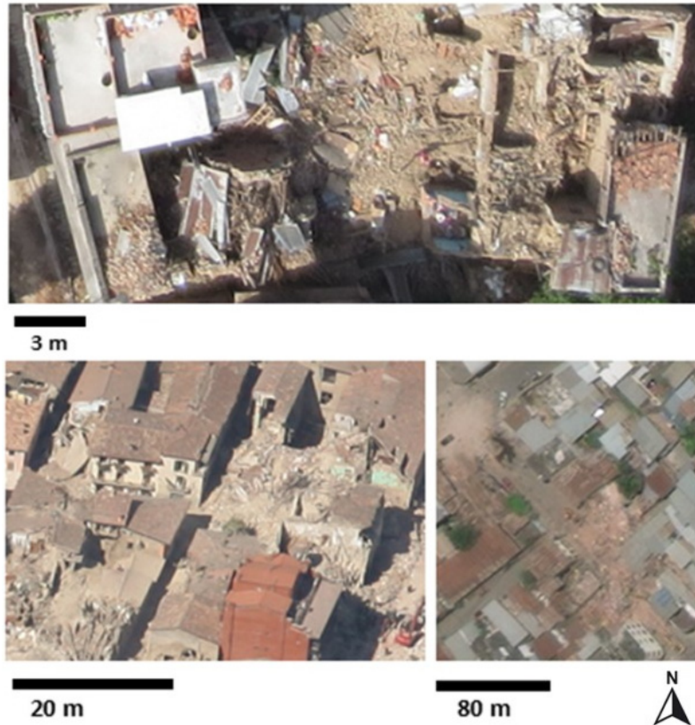
Figure 13. Examples of damaged and undamaged regions in remote sensing imagery. Nepal (top), aerial (unmanned). Italy (bottom left), aerial (manned). Ecuador (bottom right), satellite. These image examples also contain the type of damaged considered in this study: debris and rubble piles.
