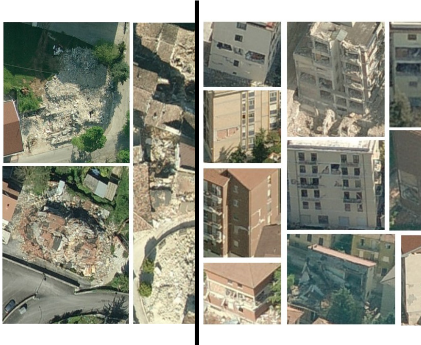
Figure 43. Examples of nadir images depicting rubble piles and debris, left. Damaged façades shown in oblique imagery, right.
