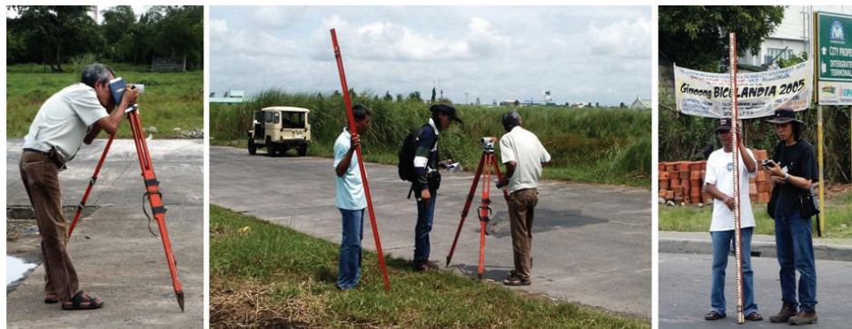
Figure 7.4 Data collection on elevation points within Naga using geodetic levelling (Photos by Rahman, 2006)
