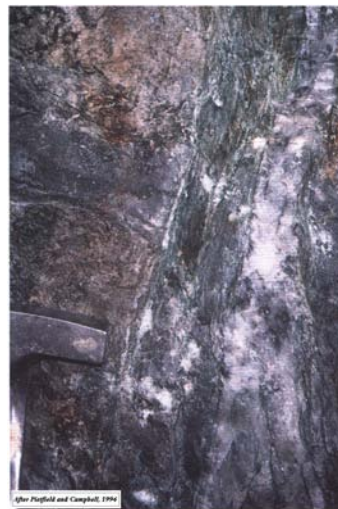
Figure 3.4: Banded replacement style mineralization within amphibolite facies alteration assemblages, Venus ore-body, Acturus mine, Zimbabwe.
