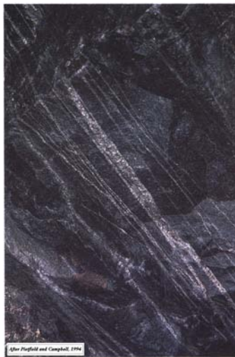
Figure 3.6: Banded sulphide and quartz replacement mineralization in Shamvaian sediments, Kimberley Mine, Zimbabwe.
