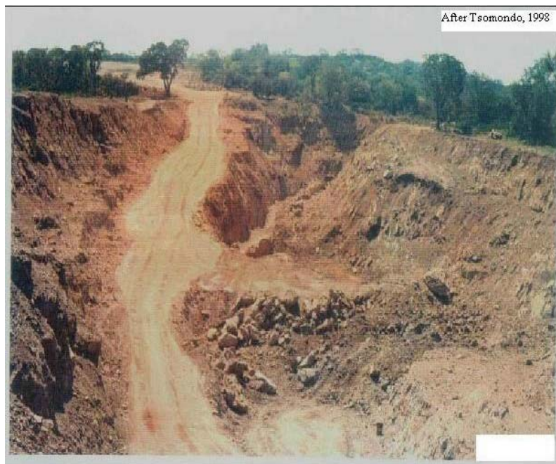
Figure 3.7: Motapa Mining Lease, Club Section Pit, looking east at the access ramp and the ore that is remaining the pit. Note the contrasting soil color marking the contact zone between the basalts and andesites.
