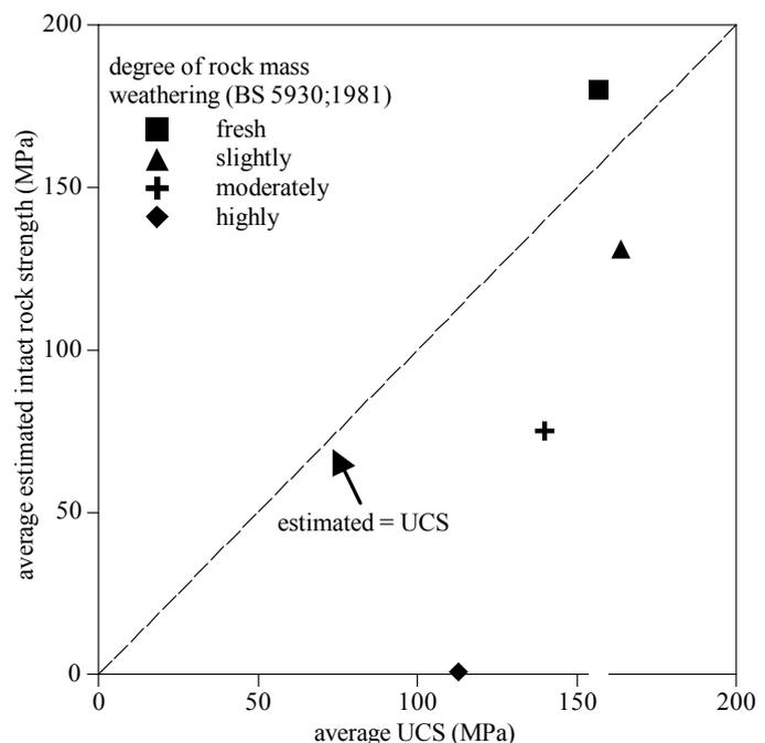
Figure 2. Average estimated intact rock strength vs. average UCS for granodiorite units with various degrees of rock mass weathering.
