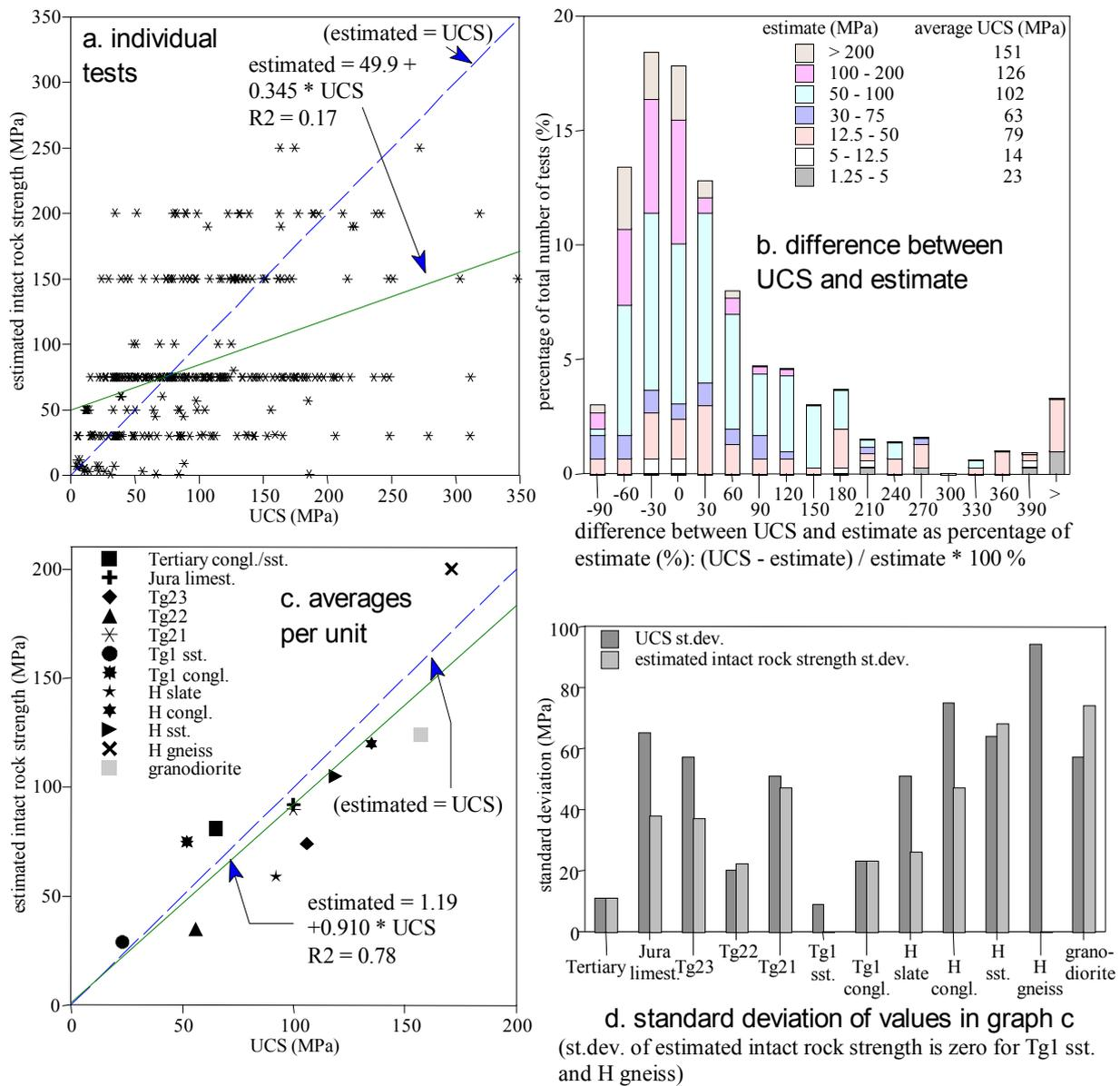
Figure 1. Estimated intact rock strength vs. strength values determined by UCS tests. (The dashed lines in A and C indicate the relation if estimated strength equals UCS strength.) (Number of UCS tests: 941)
