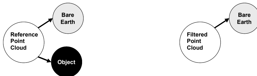
Figure 5.1 (Left) Reference data contains both Bare Earth and Object points, (Right) Filtered data only contains Bare Earth points
