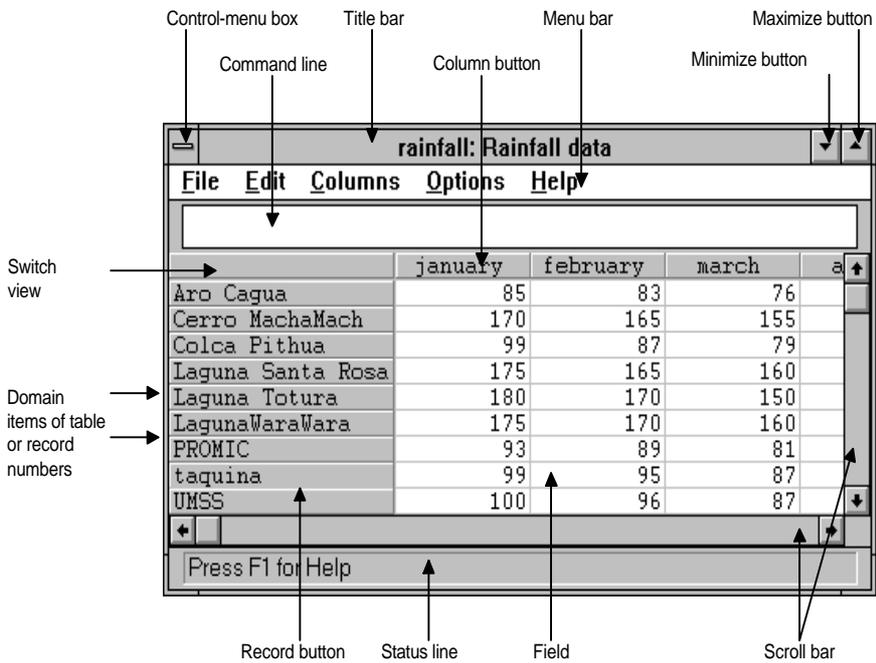
Figure 2.3 Example of an ILWIS table window.
