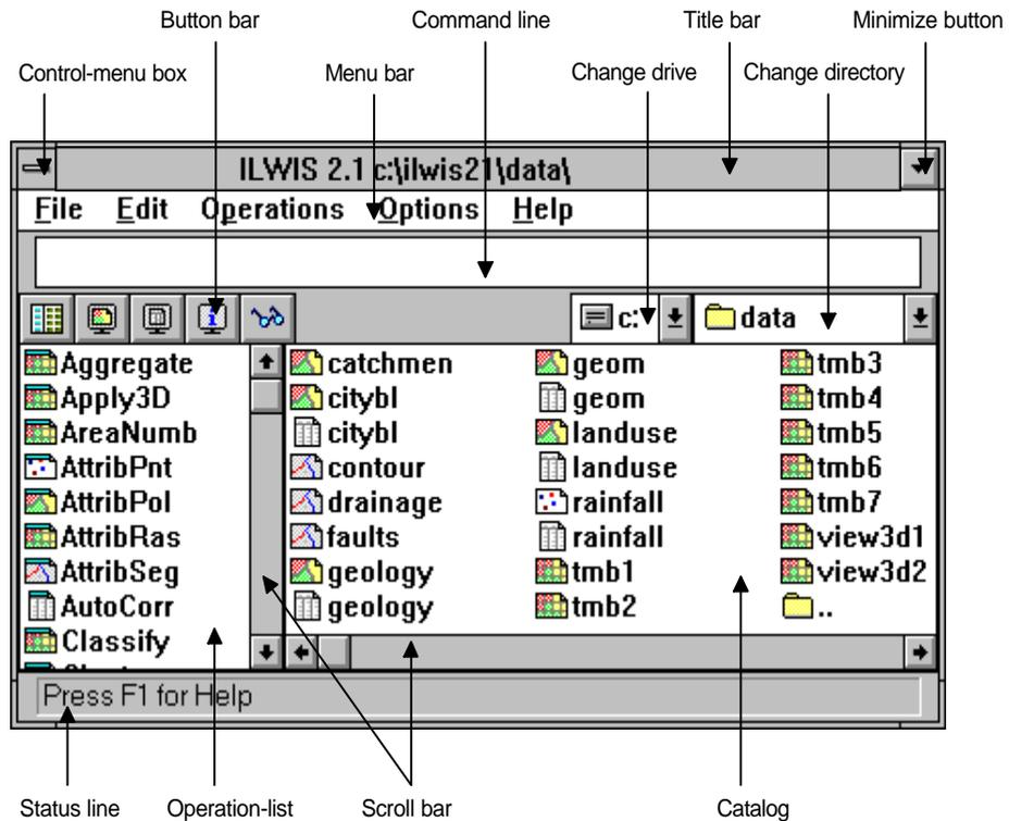
Figure 1.1 The ILWIS Main window (in Windows 3.1).
