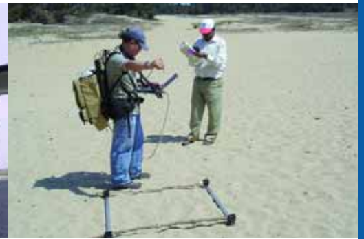
Hyperspectral field measurement (using an ASD) of the Kootwijk sand area used for the calibration of the hyperspectral air- and space borne images
