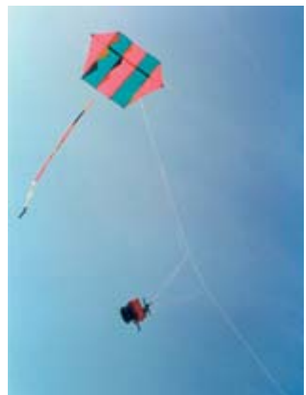
View of the kite with the rig attached to the kite line; the rig holds the camera and the radio control
