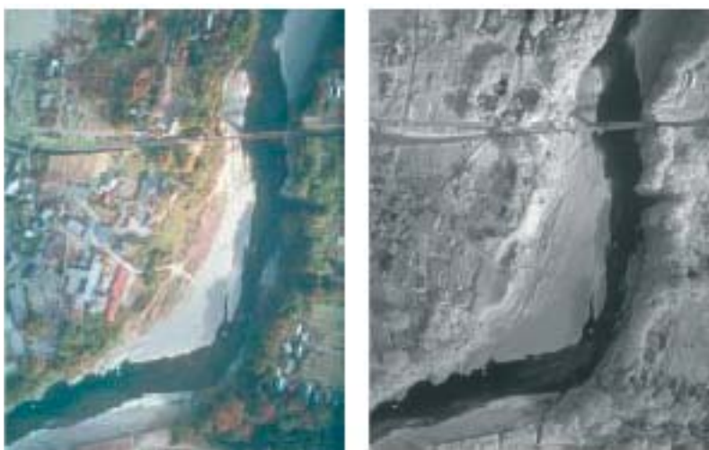
Figure 5 Color image (left) and NIR image (right) - (The NIR image distinguishes more vegetation area - upper-middle - along the river than the color image)
