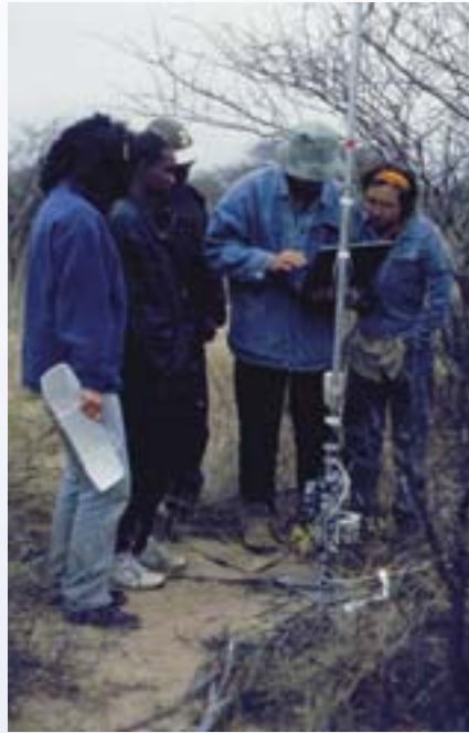
Testing to see if all sensors for sap flow measurements are properly connected
