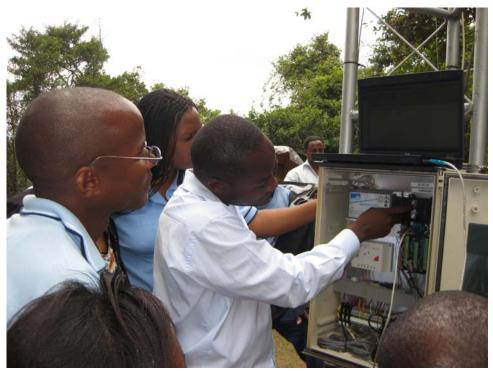
Figure 2: Reading out the logger of the climatological tower installed at the Nyungwe National Park Headquarter.
