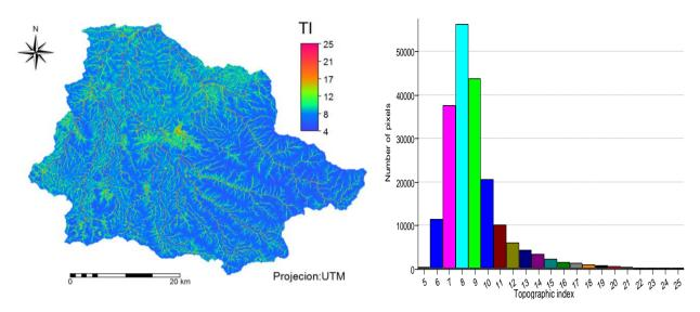
Figure 4-13: Topographic index map (left) and topographic index value distribution histogram (right)
