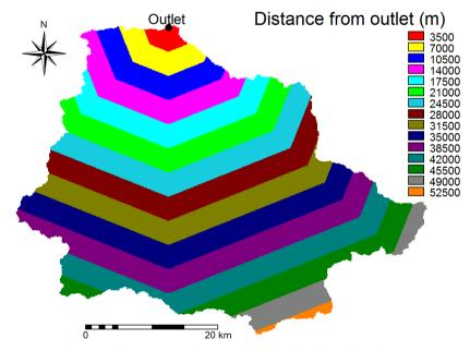
Figure 4-14: Distance area map for channel routing
