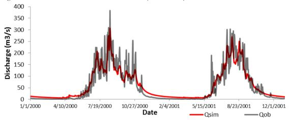
Figure 5-15: Calibrated result of the catchment (2000-2001)
