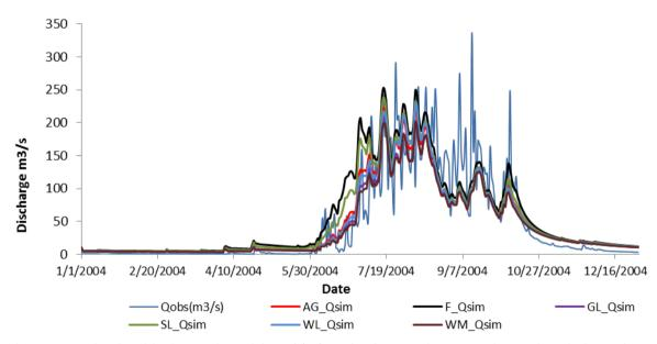
Figure 5-23: Simulated hydrograph applying ETa from land cover classes treating as the whole catchment.
