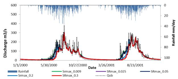
Figure 5-13: Sensitivity of the model to the changes in SRmax parameter (2000-2001)
