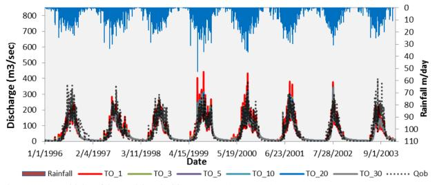
Figure 5-10: Sensitivity of the model to the To parameter (1996-2003)
