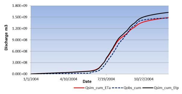
Figure 5-19: Cumulative discharge using ETa from SEBS and ETp in TOPMODEL simulation
