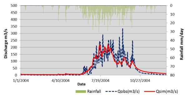
Figure 5-17: Simulated hydrograph using ETa from SEBS
