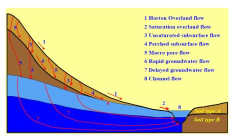
Figure 3-1: Runoff processes at the hill slope (After Rientjes (2010))
