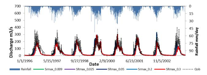
Figure 5-12: Sensitivity of the model to the changes in SRmax parameter
