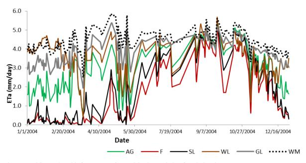
Figure 4-10: Time series ETa from SEBS after applying interpolation for missing day
