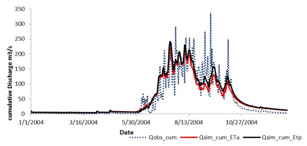
Figure 5-18: Simulated hydrograph when using ETa and ETp
