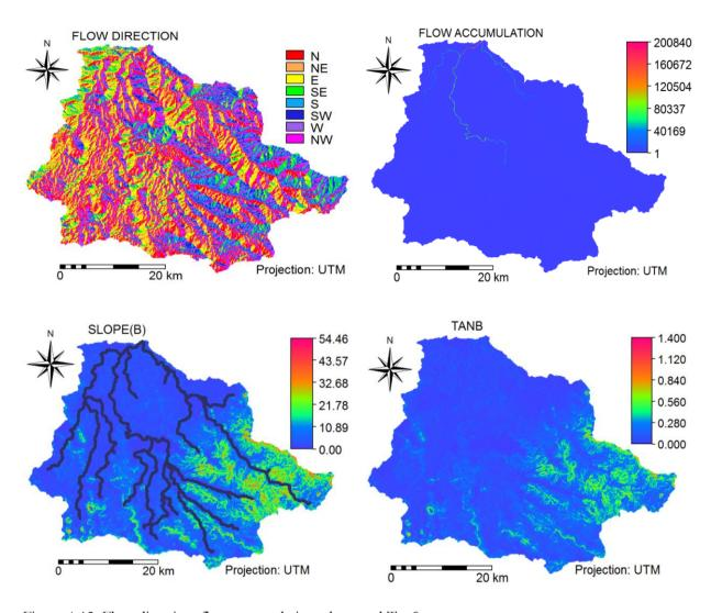
Figure 4-12: Flow direction, flow accumulation, slope and Tanβ maps
