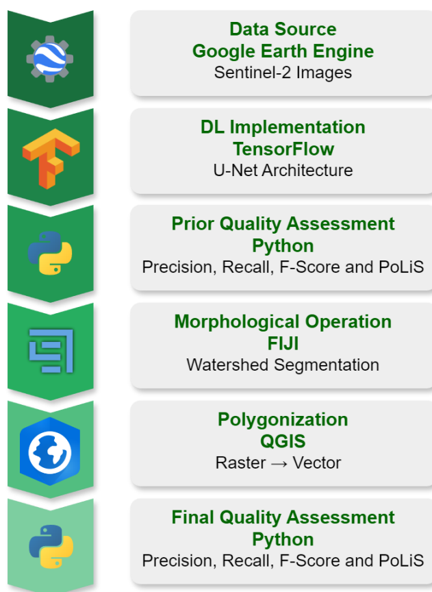
Figure 1. The overall workflow of the prototype. For each stage, the platform used is reported.
