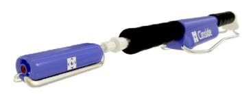
The RobotRadar is a miniaturized Doppler radar system and one of several sensors integrated in the INACHUS Robot by the partner SINTEF. The robot is intended to crawl into the
