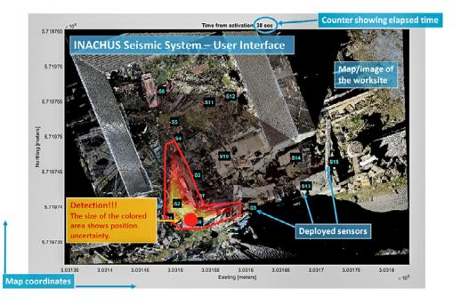
acting as a victim in the tunnels underneath the debris. A large power generator was placed on a concrete slab on the rubble to test and demonstrate the system's ability to detect signals even in the presence of very strong background noise.
