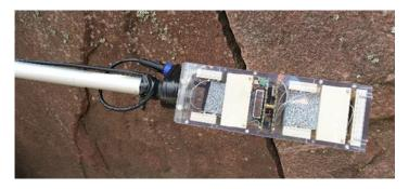
The INACHUS Robot and the RobotRadar were developed during the same period and a mock-up for the robot was needed to be able to test the radar before the robot was available. This special testplatform was further developed to a new product, the StickRadar. It consists of the same radar system as in the RobotRadar, but instead of a robot it is mounted on a telescopic stick and it will as well as a front looking camera to assist the operator.
