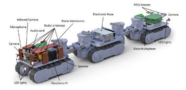
have its own OCU, a ruggedized tablet computer, making it a standalone system. Additional features include sensitive accelerometers to sense knocks from victims or other vibrations in the construction
