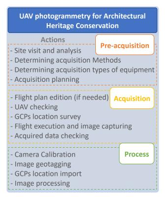
Figure 4 UAV Photogrammetry for Architectural Heritage Survey Research Activity
