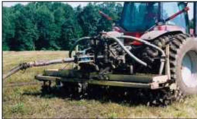
The AerWay is used to inject manure, fed to the system by a drag hose, into the ground.
