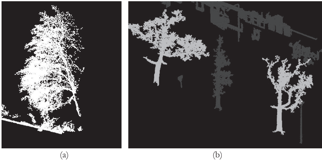
Figure 5-2: Missing tree detection analysis, (a) one missing tree hanging in the air (b) one missing tree
