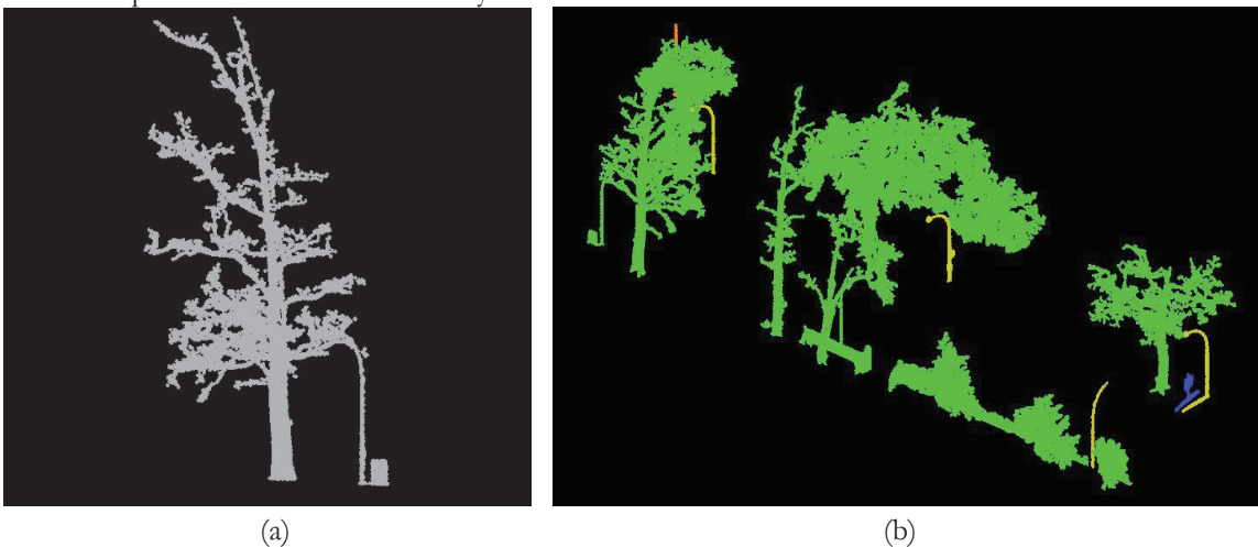
Figure 5-4: Missing lamp post analysis, (a) one missing lamp post (b) regular distributed lamp posts
