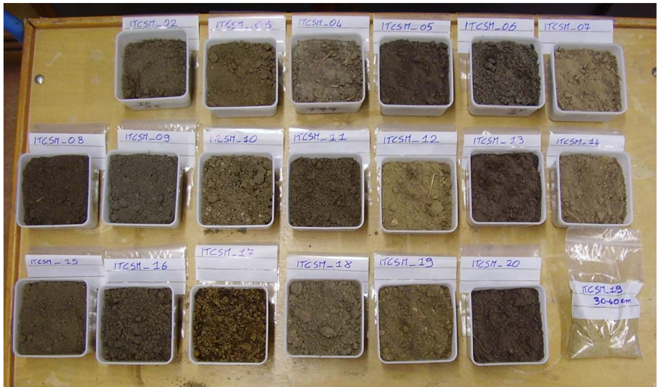
Figure 7 Soil samples collected at each site between 5 and 20 cm depth.
