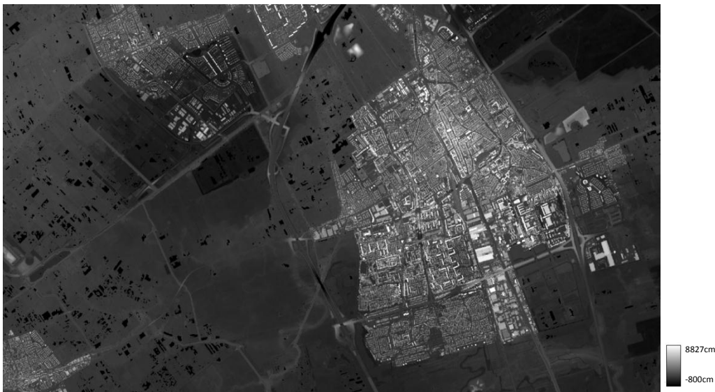
Figure 3-4: AHN-1 data (Delft area)
