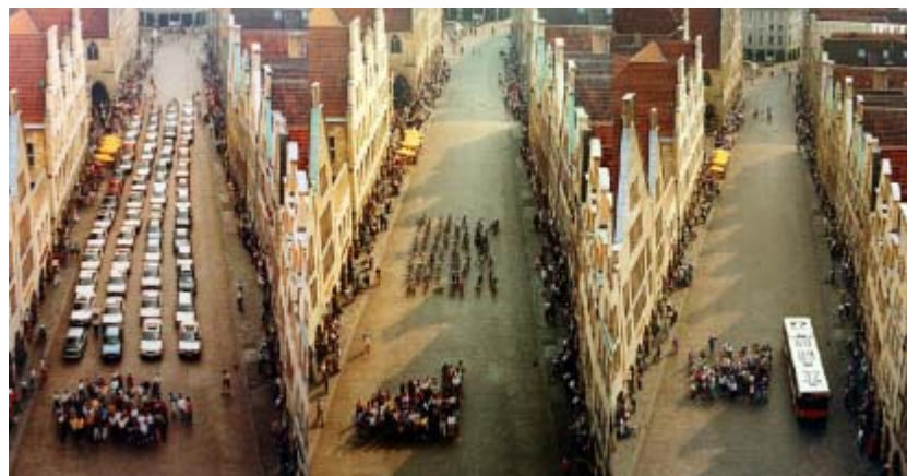
Figure 2-1 Required vehicles for transmitting same amount of passengers (Cited from (Wright and Fjellstrom 2003))
