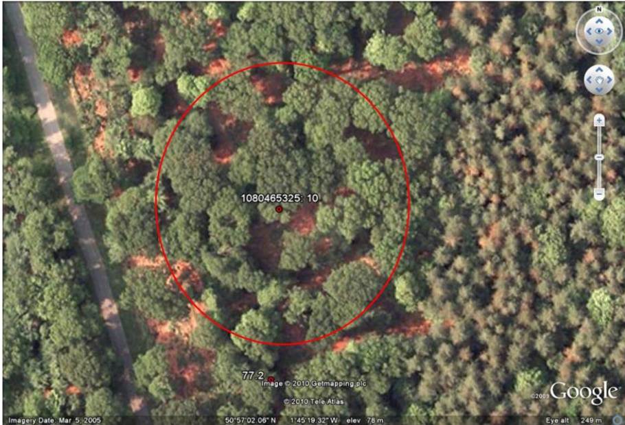
Figure 4.8: Footprint location of waveform (in Figure 4.7). Red dot shows the footprint centre, labelled with record and shot number. Image taken from Google Earth (NOAA, 2009).
