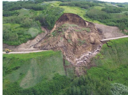
Figure 3: Schematic view and photo of a translational slide in Canada (Highland et al. , 2008)
