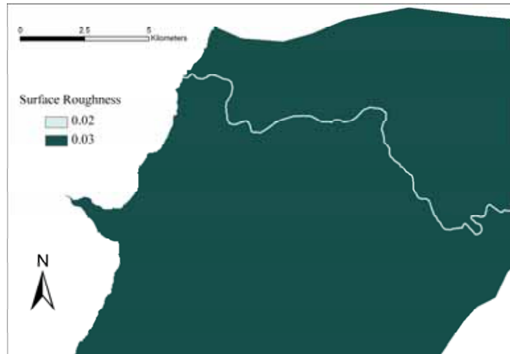
Figure 3-3: Surface roughness layer used to setup the model.
