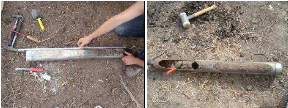
Photos B-4 – Topsoil thickness measurement (left) and sampling in the gauge (right)
