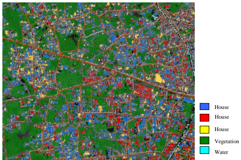
Figure 5.5 Object-oriented classification in level two. Blue, red and yellow are the type of houses; green is vegetation area and bright blue is water body
