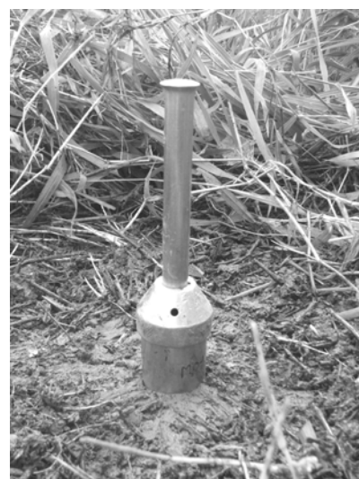
Figure 5-1: Undisturbed soil core sampling.
