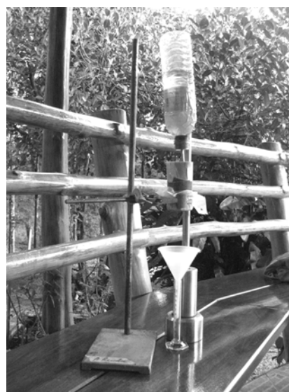
Figure 5-2: Measuring K_{sat} values in the field.
