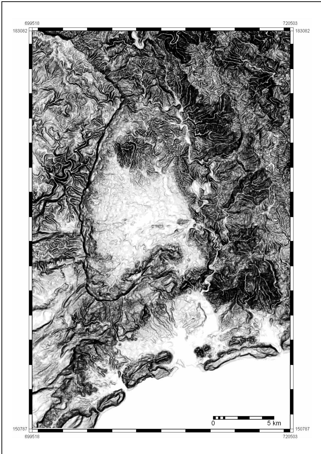
Figure 5-17. Slope gradient map stretched with histogram equalization into 20 intervals and displayed with a gradual greyscale from white (lower values) to black (higher values). Extracted lineaments from this map result in the most accurate with respect to geological truth map.
