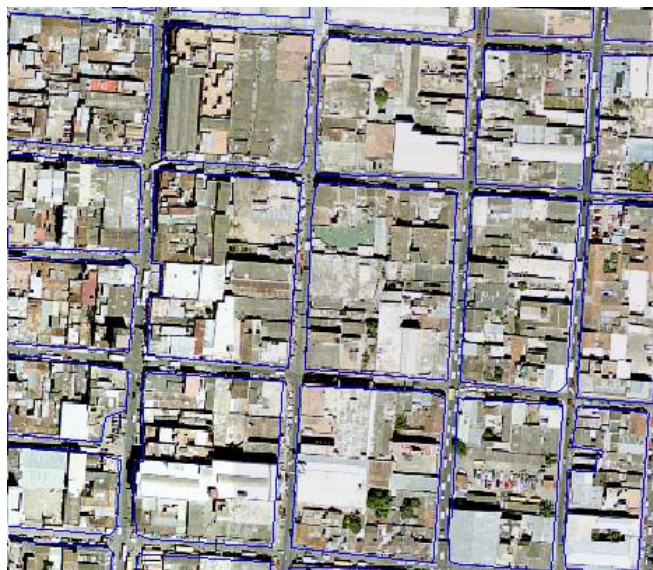
Figure 4-9: Buildings extracted from the LIDAR DEM overlaid over an orthophoto of the city.
