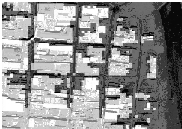
Figure 5-10: Propagation of flood over streets for buildings as solid objects (Black colour is for water)
