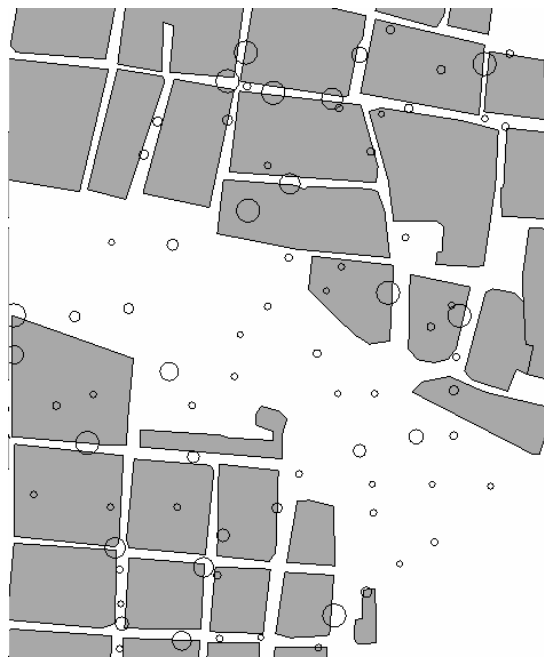
Figure 5-2: Spatial distribution of the error in elevation using a bilinear resampling.
