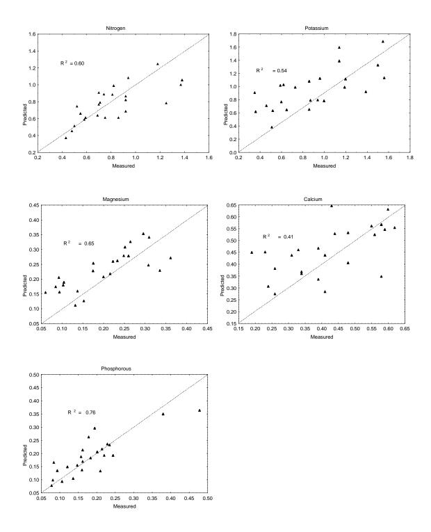
**Figure 4**. Measured versus predicted biochemicals using CRDR. A randomly selected test data set (n = 24) was plotted against biochemical concentration estimated using regression equations developed from the training data set (n = 72).
