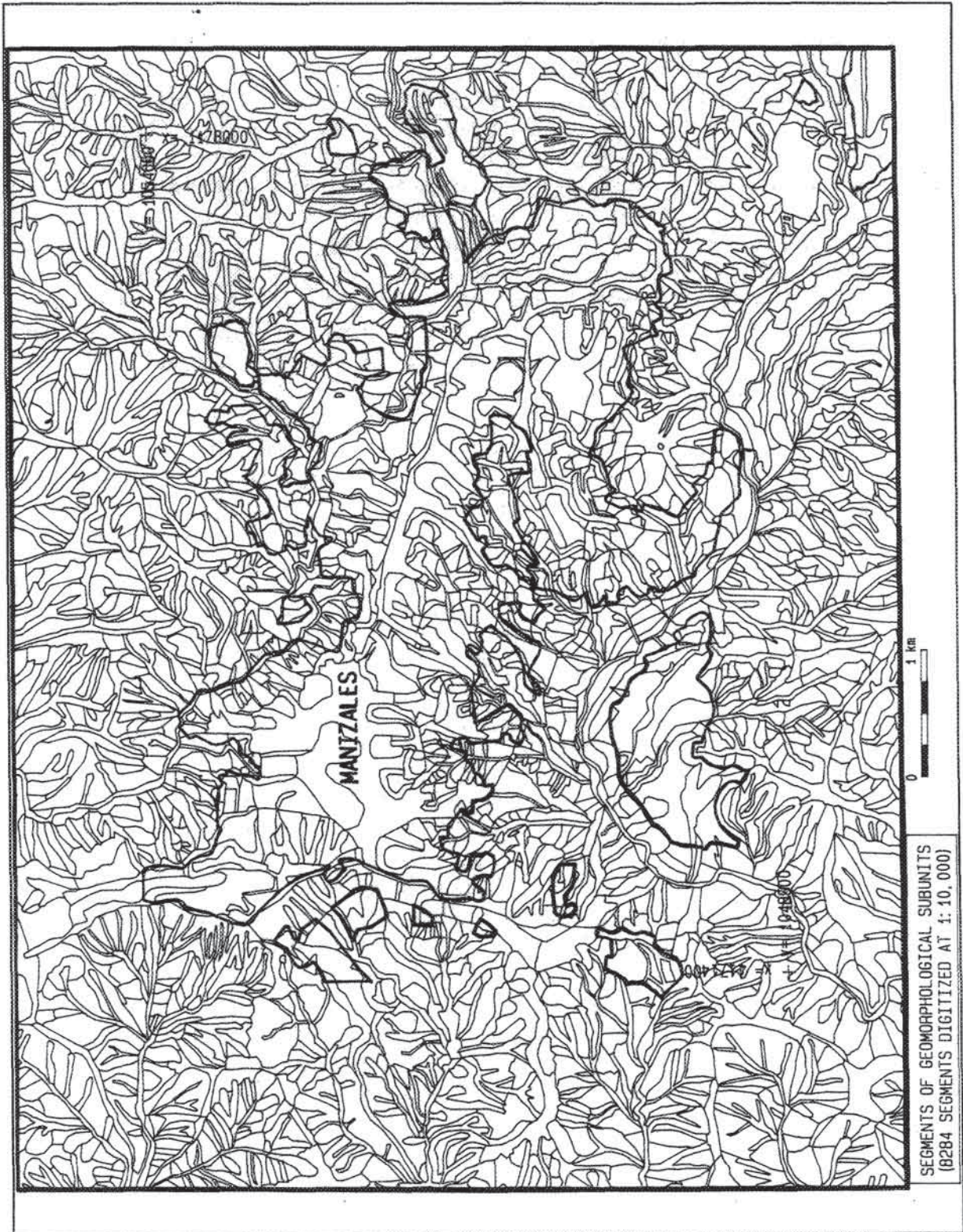
Figure 5.1: Polygon map of geomorphological subunits for the Manizales area, digitized at a scale of 1:10,000. Only the vectors are shown to illustrate the complexity of digitizing the map.
