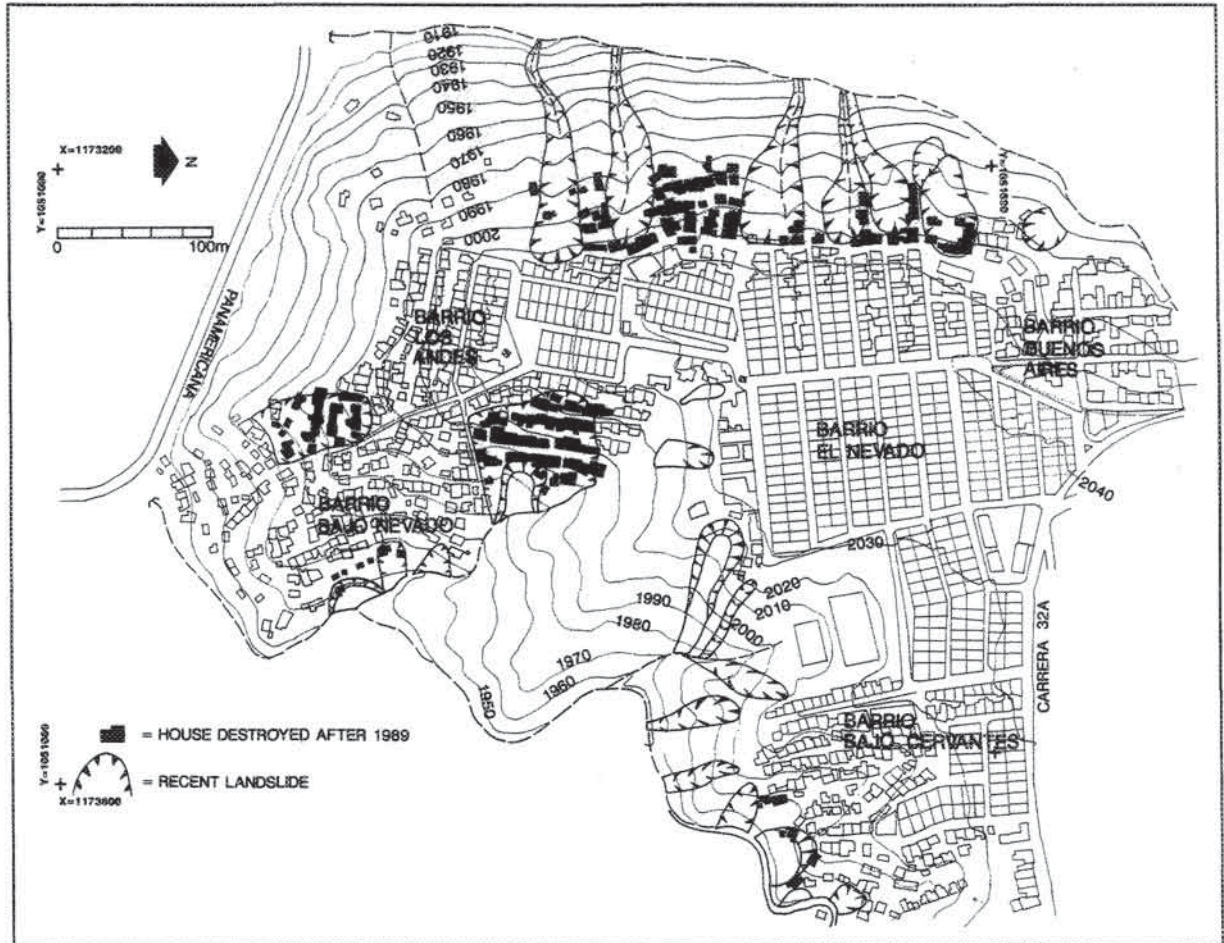
Figure 3.29: Houses destroyed or evacuated due to landslide problems in the southern neighbourhoods in Manizales.
