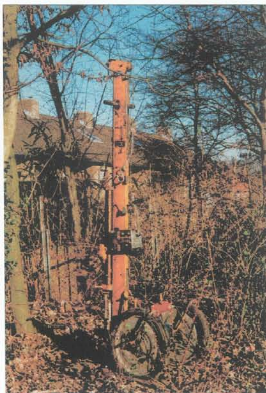
Figure 4.2: Light Dynamic probing Test in Heerlen
