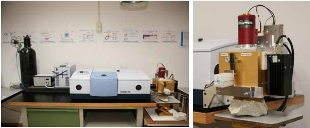
Fig. No. 29: Bruker Vertex 70 FTIR (2007) with the new liquid nitrogen cooled The thermal range of ITC's Laboratory
