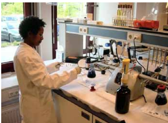
Fig No. 3: Ms. Fekerte Yitagesu, PhD researcher ESA Dept. determining the swelling clay capacities of her soil samples from Ethiopia using the methyl blue method as part of her research on the estimation of swell-shrink parameters by RS methods.
