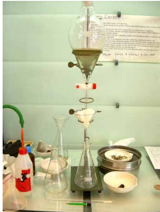
Fig.No. 25 : Heavy mineral separation using high density liquid allowed separation of specific ore minerals
