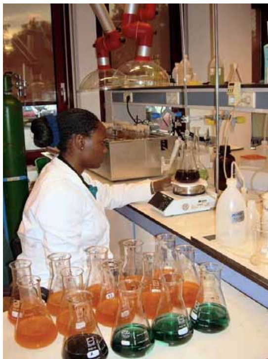
Fig.No.15: Ms Fransiska Gamises , AES-MSc student determining total organic carbon content in soils using the Walkley-Black method
