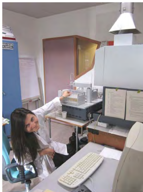
Fig. No.8 : Ms. Mila Luleva determining Na, K, Mg and Ca in her erosion soil samples from Limburg, the Netherlands with the ICP-OES
