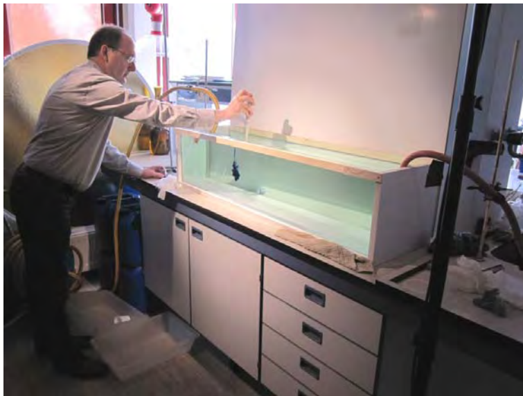
Fig. No. 24: Dr. Mannaerts experimenting how to demonstrate the salt dilution experiment for the determination of the flow capacity in a stream. This demonstration is set on video by Ms. C. Plomp with help of Mr. J. Duim for use in distance education.
