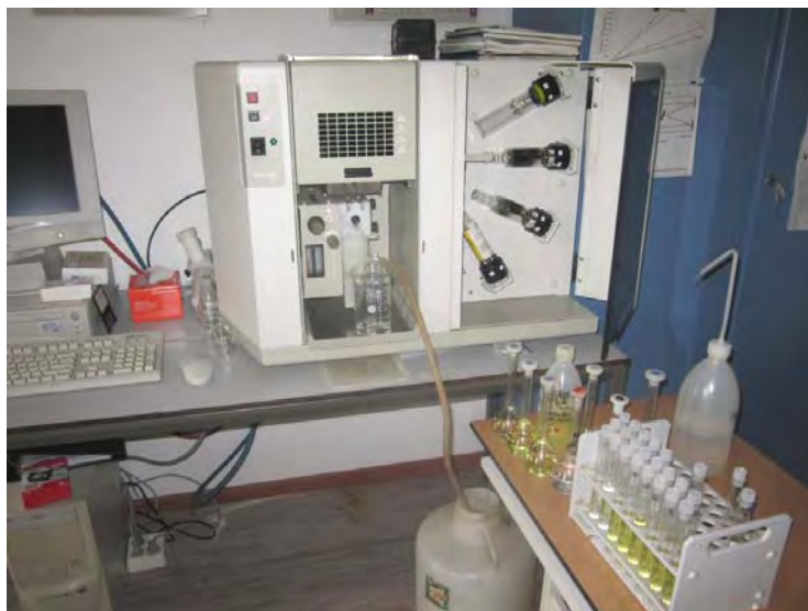
Fig.No.19: The Varian Flame AAS now operational in the GS-lab.
