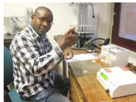
Fig. No. 11: Mr. Mustasa determining the dew point potential of his soil samples using the WRS Decagon instrument
