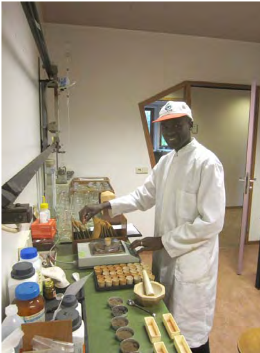
Fig. No.14: Mr. Wyclife (NRS) preparing his soil samples for carbon determination by ashing
