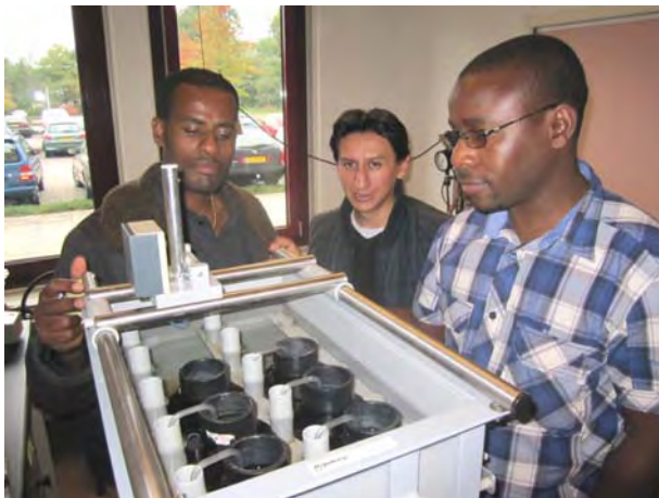
Fig.No.10: Mr. Deme, Mr. Cisneros and Mr Mustasa... measuring hydraulic conductivity on undisturbed soil samples from Salamanca, Spain
