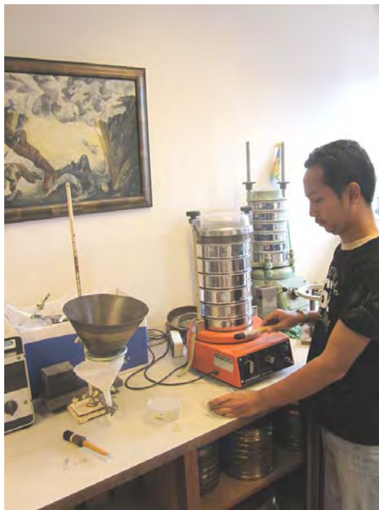
Fig. No.17: Mr. Andy Moutasim sieving his Crete beach samples of sea turtle nesting beaches
