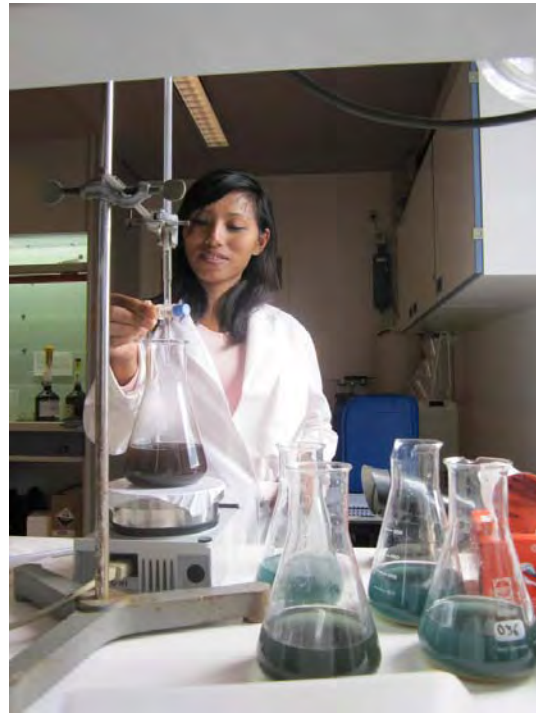
Fig. No. 15: Ms. Upama (NRS) using the Walkley Black soil organic carbon determination method
