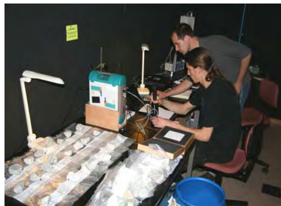
Fig. No.2 : Mr. Marinus Dalm from Delft University measures together with Dr. F. v. Ruitenbeek using the ASD IR spectrometer on Cu ore boulder samples from Chili
